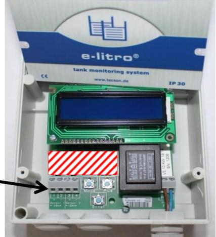
Rightmost clamping block: AC 230V N/L supply
