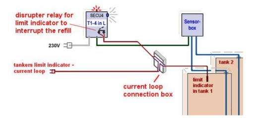
The data line from the sensorbox to the displaying device (three-pole) is prolongable up to 50m The use of a current loop connection box is optional. Therewith the tank filling can be interrupted automatically.
