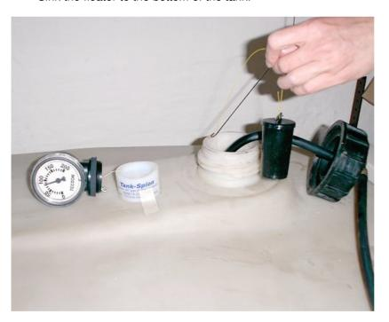
(6) Screw the dislaying unit into the affixed attachment part. Set the scale to the current level.
