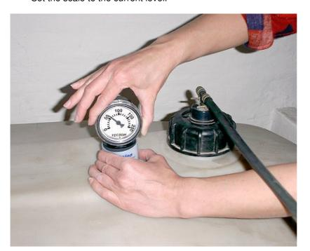
(  ${\bf 7}$  ) The mounted Tank-SPION CLASSIC shows the current tank level in cm scale units.
