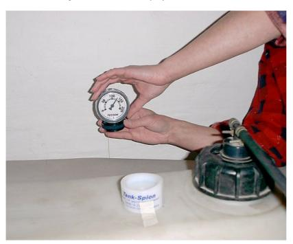
(5) Pull through the filament and mount the floater at the filament. Sink the floater to the bottom of the tank.
