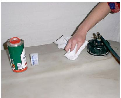
(2) Apply the special glue and affix the attachment part on the tank surface.
